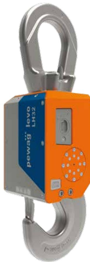
The pewag **levo hook LH32** comes with an additional brake that prevents the hook from automatically lowering when the hook is open. The optional magnet enables lifting of ferromagnetic materials weighing up to 12.5 kg. Furthermore, the placement of the magnet allows for effortless central positioning of the load.
