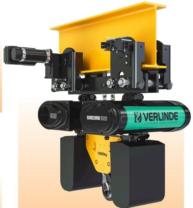
► Combined hoist for increased capacity up to 10,000 kg coupled to motorized trolley on I beam.
