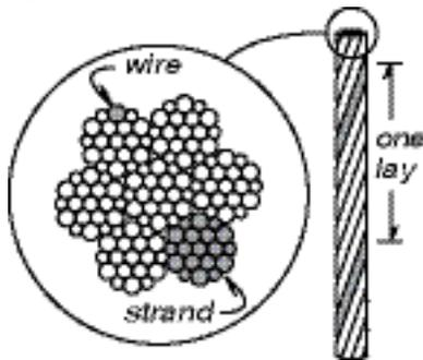
*Wire rope assembly must be replaced if more than 6 wires are broken in one lay, or if more than 3 wires are broken in one strand in one lay.*
