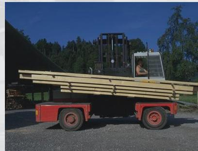
When used in combination with KOOI-REACHFORKS® (hydraulic extendable forks) the Single Height Shift System (SHSSL) can be operated for one sided loading and unloading but also one of the hydraulic forks can operate independently. Which makes the forklift truck much more flexible.
