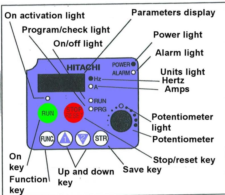
Setting of the current limitation via the speed inverter SJ200 :
