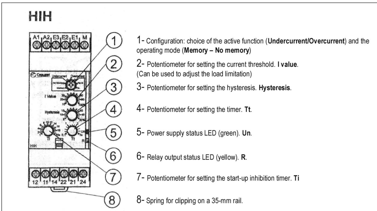
The load limiter is adjusted in the factory to the value of about 110% of its MCU.
