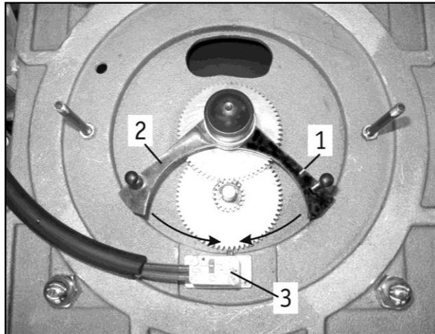
Type with IP65 cam: Remove the protective cover of the device, the cams (1) which are now accessible can be positioned with the help of a worm (2) using a screwdriver.
