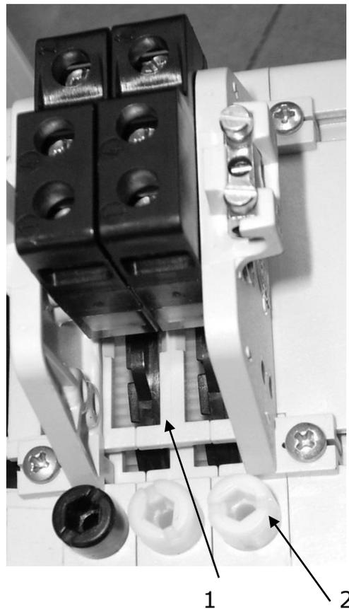
Each adjustment screw (2) corresponds to a TOP or BOTTOM limit position.
